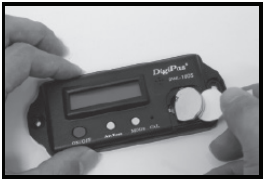
For the first time usage, remove the plastic strip to connect the battery
