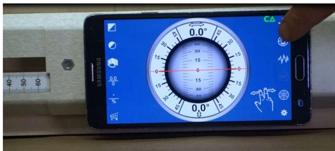
6. The bike does not have to perfectly vertical for accurate measurements but should be within 5 degrees of vertical for best results.
