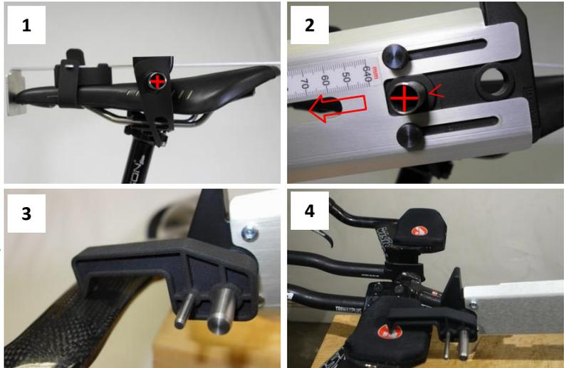
4. TT pad location can also be recorded. It can either be entered in the App in the 'Handlebar' field, or as a User-Defined measurement. In the Handlebar field a calculation from the BB will be made. Enter a "Thickness" of 1mm for a BB-to-TT pad surface measurement.
